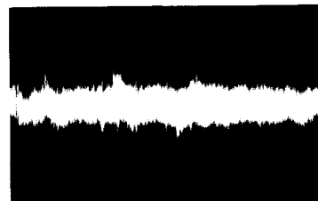
Focus signal P108 pin 2 V: 10mV/div H: 0.5mS/div
